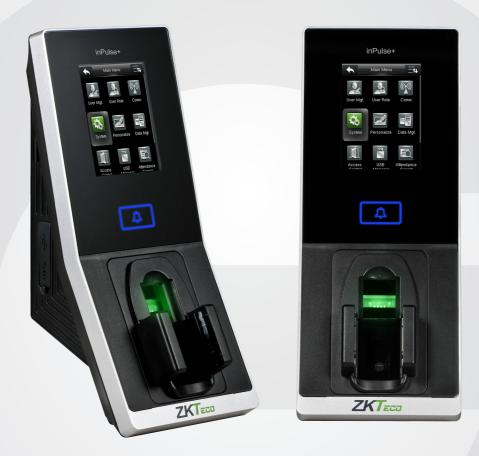
inPulse+ is a multi-biometric reader capable of capturing and processing finger vein and fingerprint biometric data at the same time. Ergonomic, intuitive and highly secured, inPulse+ leads us to a new era of enhancing security with biometrics. Its infra-red rays illuminate the vein pattern which is then converted into a biometric template. Both the vein and fingerprint templates are then stored in the database for subsequent matching.
